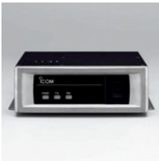
UR-FR5000 (VHF) / UR-FR6000 (UHF) Channel module units
