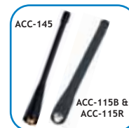
UHF Antenna 6", 450 - 490 MHz, SMA (ACC-145) & VHF Antenna 6", 148-162 MHz & 162-174 (ACC-115B & ACC-115R)
